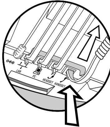
2. On the back of the phone, remove the key located behind the hookswitch and reposition it so that the end tab (at a 45° angle) is facing up.
