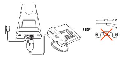
**IMPORTANT** Use configuration **A** on the bottom of the base, which works for most phones including Cisco phones.
