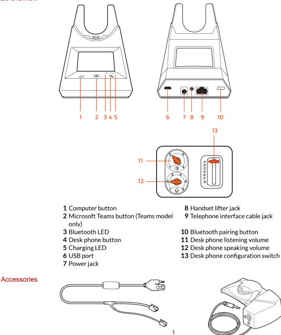
**1Electronic hookswitch cable (EHS cable)** Electronically and automatically answers/ends a desk phone call. Enables remote call control with your headset.
