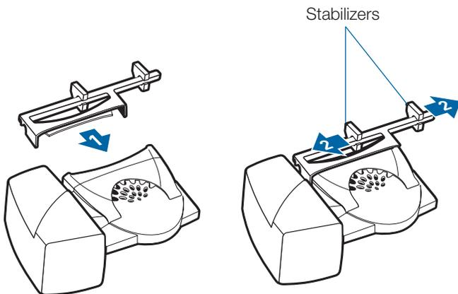
Use extender arm when the handset lifter needs additional stability lifting and returning handset to cradle.
