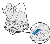
Use the speaking volume major adjust control on the bottom of the base for large incremental adjustments.
