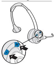
Push on the "+" and "-" buttons to adjust listening volume in minor incremental adjustments.
