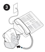
Plug the handset cord into the handset jack in the bottom of the base.
