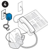
Plug the AC charger into an outlet and into the base's AC charging jack.
