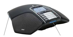
The **Konftel 300Wx** is a battery-driven wireless conference phone that can be connected to DECT systems, mobile phones or PCs. It can be connected to a Konftel DECT base station or any GAP-compatible DECT system.
