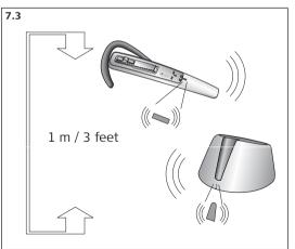
7.3 Make sure headset and base are within 1 meter/3 feet of each other. When pairing is successful, both visual indicators will flash green 10 times, and the visual indicator on base unit will turn to steady green.
