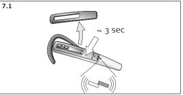
**7.1** Remove snap-on cover. Press reset button on headset for 3 sec. Visual indicator on headset will flash red/green rapidly. <sup>1</sup>
