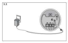
**3.3** Connect AC power adapter to port on bottom of base unit, then connect to AC power outlet. Visual indicator on base will light green.
