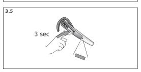
**3.5** Turn on headset by pressing answer/end button for 3 sec. (visual indicator will light green for 2 sec. and two "beeps" will be heard), or by placing headset in charge cradle. Turn off headset by pressing answer/end button for 3 sec. (visual indicator will light red for 2 sec. and two "beeps" will be heard).
