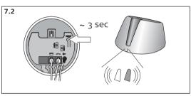
**7.2** Then press reset button on base unit for 3 sec. Visual indicator on base unit will flash red/green rapidly.
