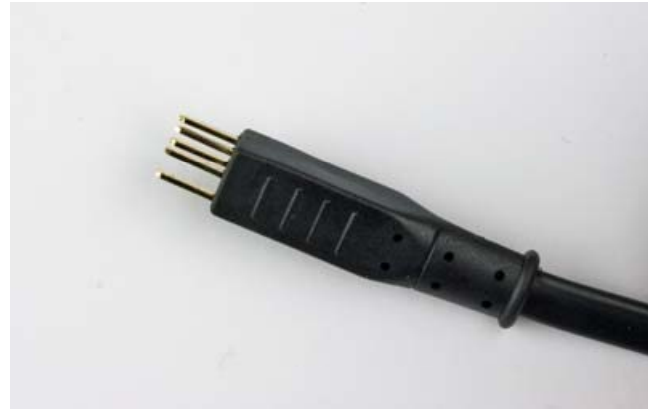
Connector; reverse side marked "TOP" (= side of connector pointing upwards at installation)
