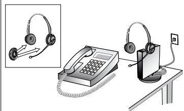
The battery in the headset is not initially charged and the battery charging indicator on the base will flash continuously during charging.
