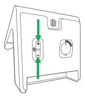
To adjust the desk phone microphone volume, press + or - buttons, located on the bottom of the base.
