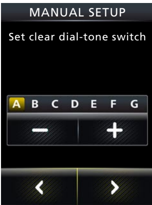
Figure 16: Manual clear dial-tone switch position selection for Jabra PRO 9465-Duo / 9470
