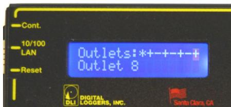
Outlet (port or relay) status shows on the first line. The outlet name or time/date of last modification shows on the second line. Three symbols are used for relay status + (ON), - (OFF), and \* (LOCKED). In this example, the relay 1 is locked ON, the even numbered relays are ON, and relays 3.5.7 are OFF. The flashing cursor indicates outlet 8 is selected:
