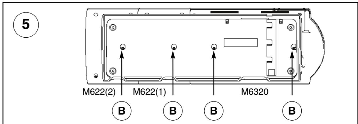
9. If you are connecting one M622 Add-On Module, position the wedge-shaped base as shown in Figure 4. If you are connecting two M622 Add-On Modules, position the base as shown in Figure 5. Align the plastic tabs in the base with the notches provided on the M622 and telephone set.
