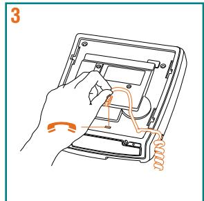
Attach the receiver cord. Route the cord in the channel.
