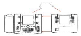
The 560M provides 10 softkeys in each column (totaling 20 keys) on the keypad. The 560M also provides 3 keys at the bottom left of the unit. These keys represent "Page 1", "Page 2", and "Page 3" of the LCD display. The 560M has 20 keys available on each page (totaling 60 softkeys). Each key provides an LED for indicating call status. The 560M provides an LCD for displaying key labels.
