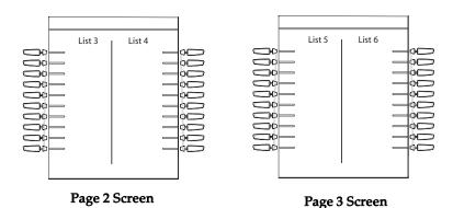
To use the 560M, press the function key for the page you want to display to the LCD (page 1, page 2, or page 3), and press the applicable softkey.
