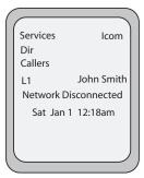
Check that the cables are tightly connected to the phone and to the wall jack. The phone should automatically detect when it is reconnected and displays the "Network Connected" prompt for a few seconds. However, if changes have been made to your phone's network settings, you may need to restart your phone.
