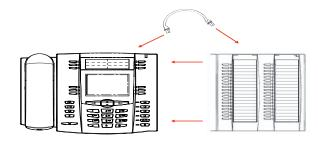
The 536M provides 18 softkeys in each column (totaling 36 keys) on the keypad. Each key provides an LED for indicating call status. The 536M provides a paper label for convenient key labeling.
