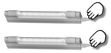
6 Locate the series of bulbs next to the non-functioning bulb, then ensure all power cords are fully inserted in place.
