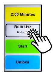
4 Plug the unit back into an electrical outlet and reset the Bulb Use Hours counter by pressing "Bulb Use" for 6 seconds. Then, enter "0 - 3 - 1 - 4" when prompted.
