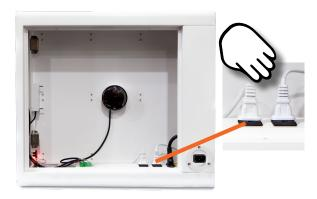
4 If more than one bulb is non-functioning, open the Removable Service Panel and ensure the white power cords are completely plugged in.
