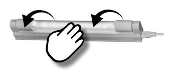
Wearing cotton gloves, rotate the bulb to ensure it is seated correctly (clicks in place).
