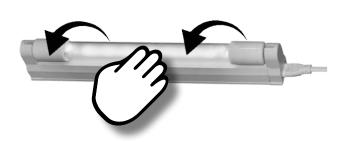
Wearing cotton gloves, rotate the old bulb counter clockwise to release it from the lamp socket. Install new bulb by placing into lamp socket and rotating clockwise until you hear a click.
